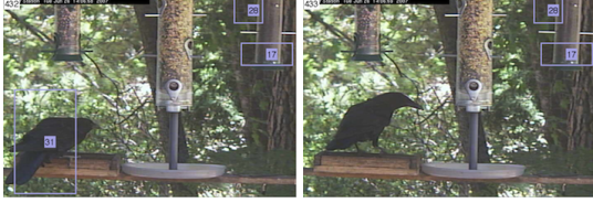
Figure 2. Mean shift fails when birds in consecutive frames move too suddenly (31) and when the appearance model contains much of the background (21 and 17), while our approach is able to recognize this two views as the same bird due to their similar appearance.
